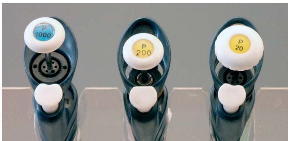
Figure 2.2: The P1000, P200, and P20 models of Pipetman® (photo by S. Dellis)
